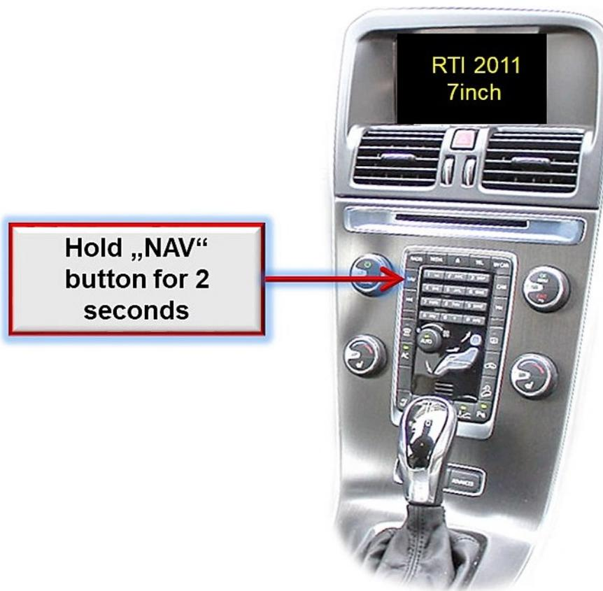
Pressing the **NAV** button on the infotainment panel for 2 seconds, switches the input from the factory video to the video source.
