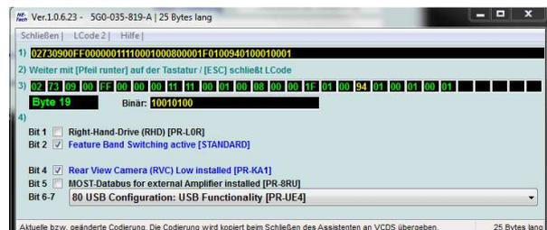
After coding, head-unit must be reset. On most head-units by long-pressing (about 20 seconds) of the ON/OFF key.
